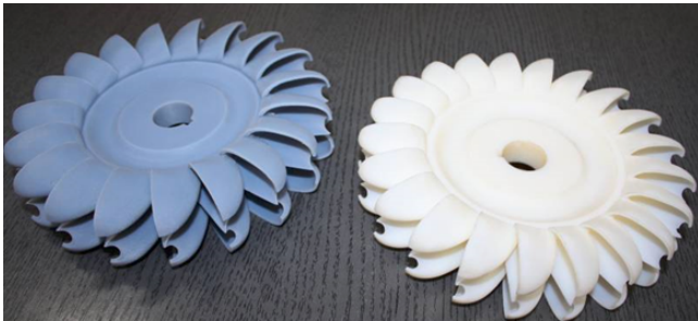
Fig. 2 The final shape of the two Pelton runners
